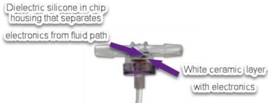
Figure 2. Photo of pressure sensor body with chip inserted
