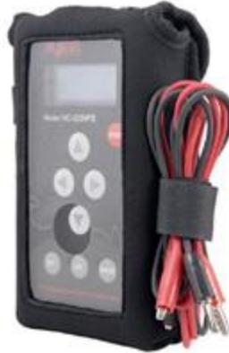
2. Measure Excitation Voltage- in addition to generating an input with a mV generator to simulate pressure, the excitation voltage can also be verified. The sensor output is in units of mV per psi per volt excitation so this voltage is an important factor in overall sensor accuracy. The voltage appears on the monitor cable pins 1 (plus) and 4 (minus):
