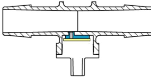
Figure 1. Illustration of pressure sensor body with chip inserted
