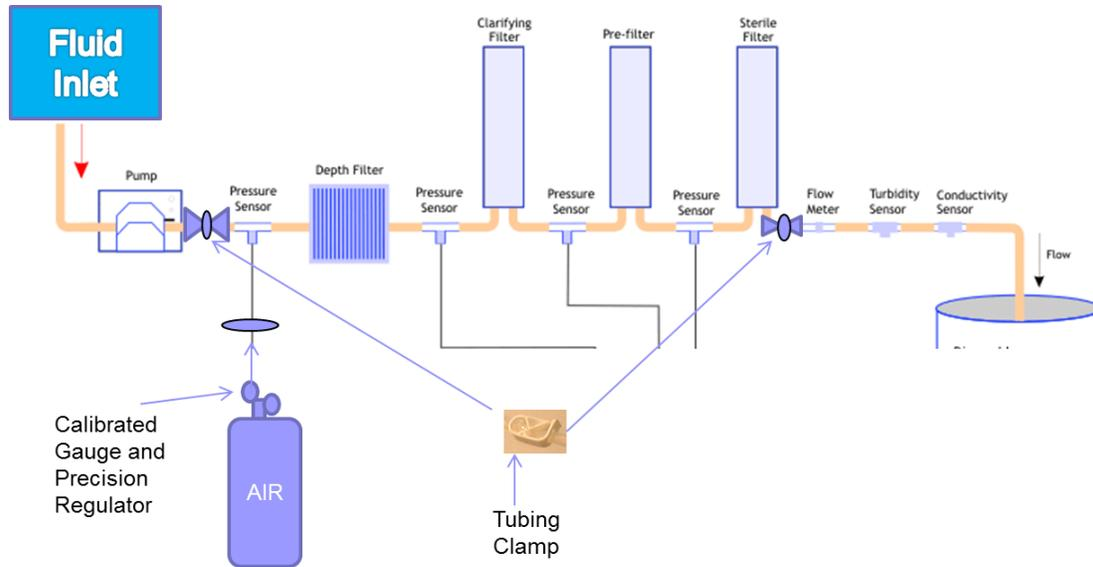
Figure 5. Illustration (for representation only) of a test set up where a calibrated reference pressure could be compared to pressure sensor readings.
