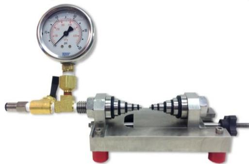
A precision regulator connected to an air source and calibrated gauge (calibrated gauge and precision regulator not shown) can be connected to inlet connection on the left side shown below. With the isolation valve open, the calibrated gauge reading can be
